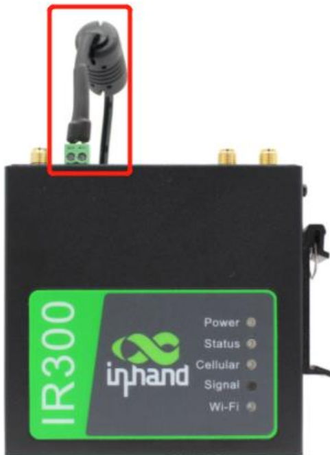
Figure 3-5 Power Supply Installation
