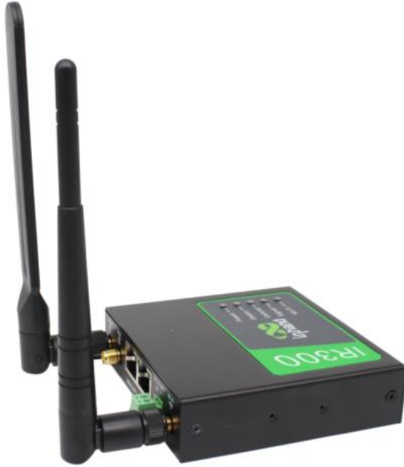
Figure 3-4-a Glue Stick Antenna Installation
